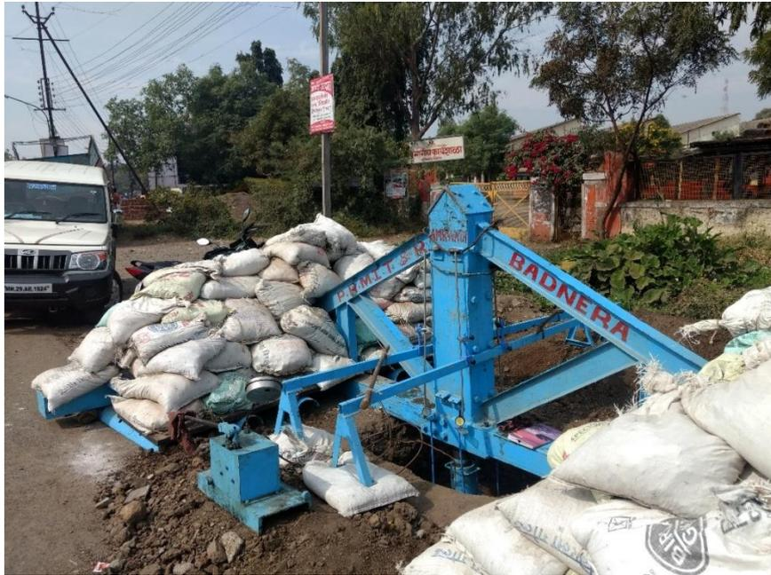
Photo: Plate load test
