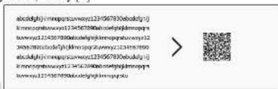
Fig. 1: Example of high capacity encoding data in QR code
