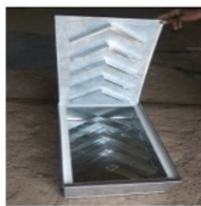
Figure 1.1 (a): Insulated Box with collector plate.
