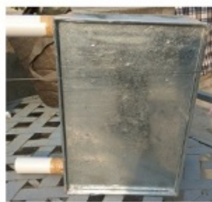
Figure 1.1 (b): Complete assembly of Solar Air Heater
