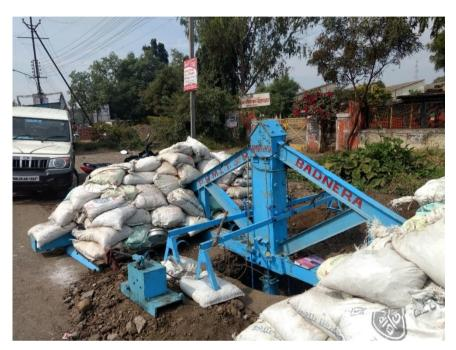
**Photo: Plate load test**
